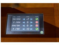
A console equipped with OrgNG3.0 system - TFT touchscreen, custom couplers configuration
