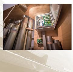
A part of the mobile, wireless pipe organ equipped with OrgNG3.0 system - division driver with a wireless transmission module
